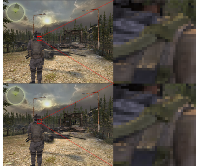
Figure 1: The Bootcamp demo from Unity3D 1 using uncompressed textures (top) and using textures compressed with FasTC-64 (bottom). The visual quality of the scene is only slightly altered and no visible artifacts appear. The scene uses 156 textures which were compressed in a total of 8.75 minutes by our method. The same textures are compressed by the BC7 Compressor in the NVIDIA Texture Tools in a total of 13.27 hours.
